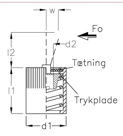
$\begin{array}{lll} d1 & = 10 \\ d2 & = M4 \\ d3 & = 10 \\ H & = 12 \\ I1 & = 12 \\ I2 & = 7.5 \\ screw driver & = GN 715.1-5 \\ Side power N at I2 = 75 \end{array}$
